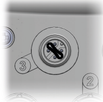
Fig. 19: Conductive rubber band in connection socket 3
