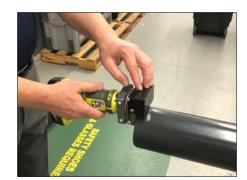
With the left hand, rotate the plastic guard up and place the tool against the pipe face with the cutting blade slightly above the pipe surface. If the blade is resting on the pipe surface when the tool is turned on, the tool will quickly jump to the right.
