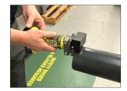
Now with the left hand, push the power on/off switch located near the base of the tool.
