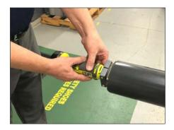
After the bevel is completed, raise the tool above the pipe surface and turn the tool off by pushing in the power on/off switch.
