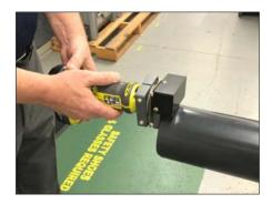
Grasp the handle with the right hand, holding the tool in line and square with pipe face.
