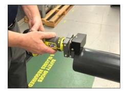
Slowly lower the tool to the pipe surface. Rotate the tool <u>counter-</u> <u>clockwise</u> while trying to maintain the tool square with the face of the pipe. Two revolutions around the pipe will produce the desired bevel. The process gets easier to perform after a few attempts.
